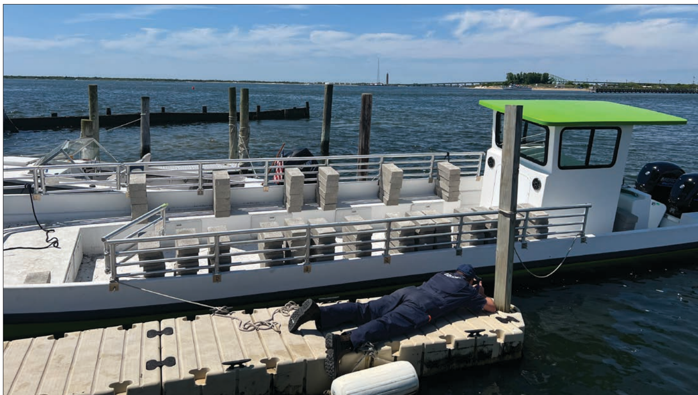
Coast Guard CWO4 Glen Browning checks measurements near Captree State Park, New York, during a simplified stability test on a new passenger vessel built by Henriksen Boat Designs. Coast Guard photo by Bill Grossman
