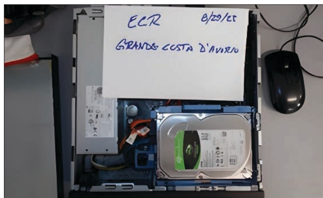
Modern ships have numerous devices, like this hard drive from the Grande Costa D'Avorio 's engine control room, that can provide information that aids investigators after an incident. Coast Guard photo
